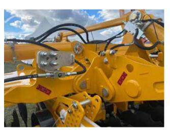
UNFOLDING SYSTEM WITH HYDRAULIC PROTECTION
