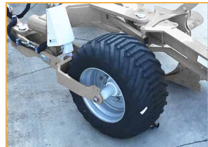
HYDRAULIC WHEEL FOR DEPTH ADJUSTMENT
